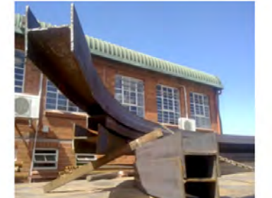
203 H BEAM ROLLED ON EDGE
